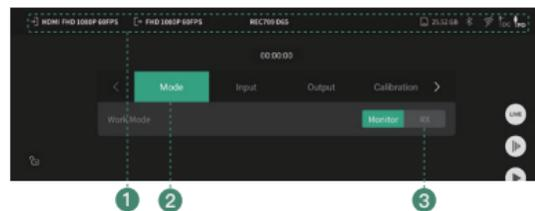
Note: Once selected, the system will prompt to reboot. After confirming, the system will reboot and switch to RX mode.
